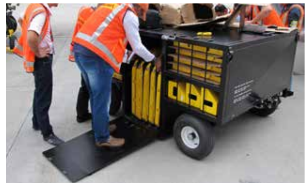
Rapidly deploy aircraft scales from transport cart with ramps, without needed to lift scales.
